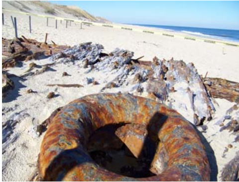
The iron hawsepipe, prominent in this picture, is where the metal chain from the anchor goes through the hull of the ship.
